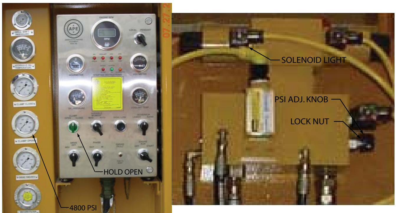
Figure 2-C. Setting Relief Valve
